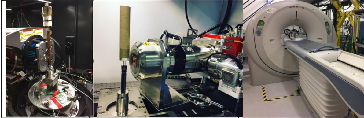
Figure 2. The multi scale X-ray imaging and experimental core flooding facility at Imperial College London with micro X-ray CT (left, centre) and medical X-ray CT (right)
