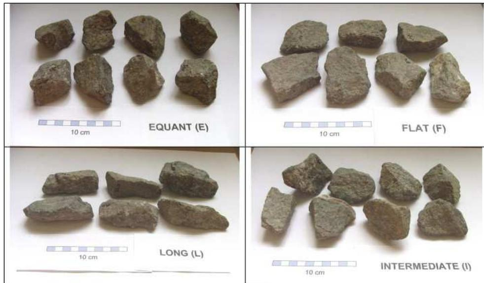
Figure A.1: **Example particles digitalised in the Shape Library.** The particles were initially classified in groups on the basis of visual criterion for the purposes of labelling them. Picture taken from [27].
